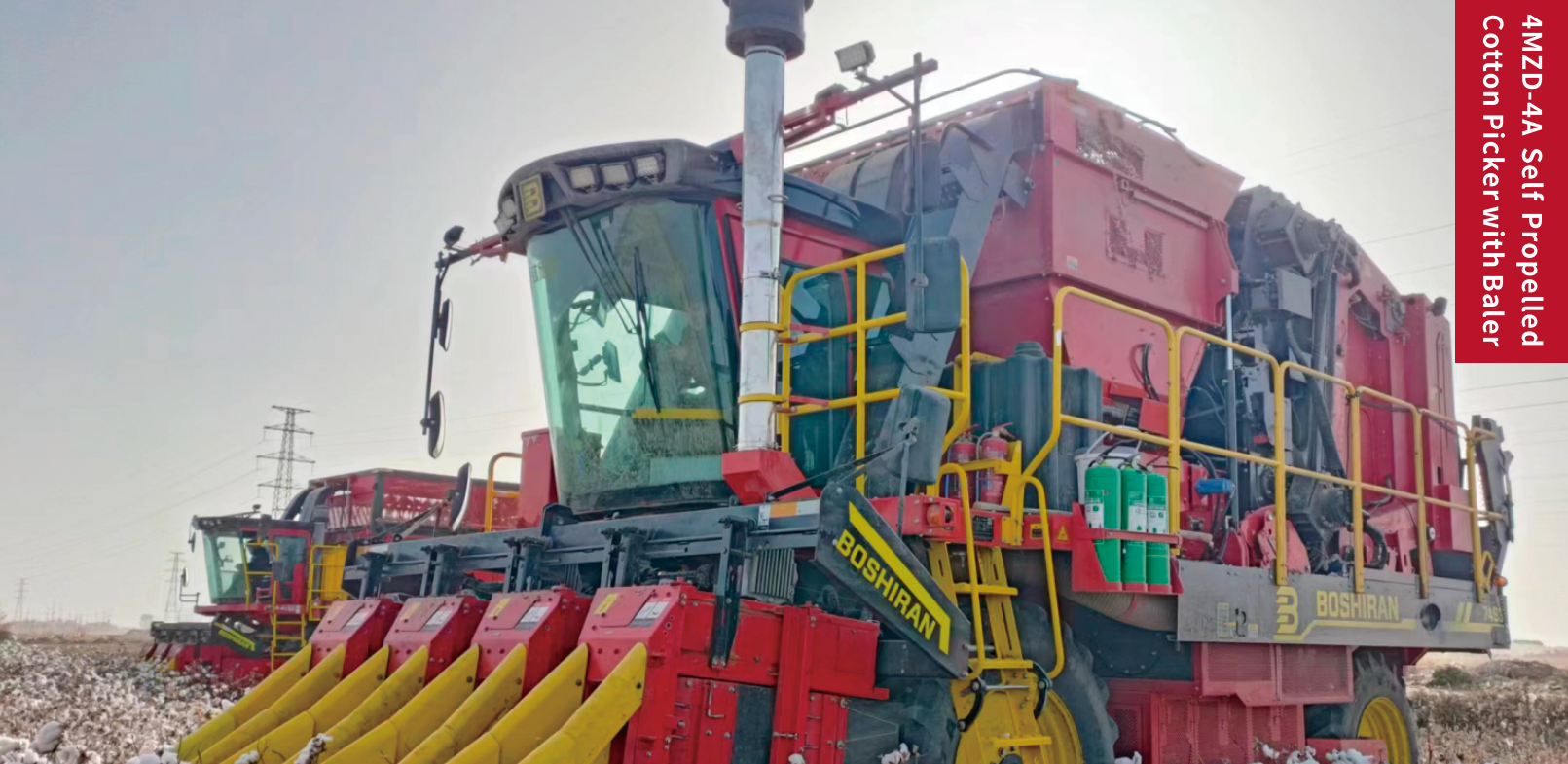
Boshiran 4MZD-4A Self Propelled Cotton Picker with Baler Independently developed and manufactured by Xinjiang Boshiran, this machine revolutionizes cotton harvesting by integrating four critical functions into a single seamless workflow: picking, conveying, baling, and automated cotton discharge—eliminating downtime and maximizing field efficiency.
