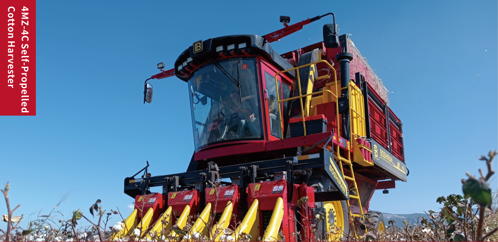
Boshiran 4MZ-4C Self-Propelled Cotton Harvester Independently developed and manufactured by Xinjiang Boshiran, this machine revolutionizes cotton harvesting by integrating four critical functions into a single seamless workflow: picking, conveying, baling, and automated cotton discharge—eliminating downtime and maximizing field efficiency.
